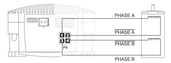
Figure 2.3.6: 4 Lead Motor Connections
